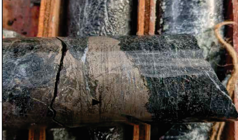
Semi massive nickel and copper bearing sulphides at 472.2m in EL-22-97b. Mineralization is hosted with well mineralized E&L gabbro with heavily disseminated to blebby, to semi massive sulphides.
