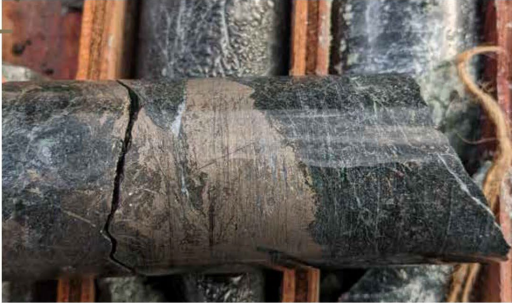
EL-22-97b 472.2m 0.29% Ni, 0.32% Cu Semi massive Po-Cpy-Pn sulphides in variable textured gabbro
