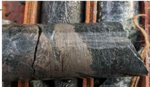
EL-22-97b 472.2m 0.29% Ni, 0.32% Cu Semi massive Po- Cpy-Pn sulphides in variable textured gabbro
